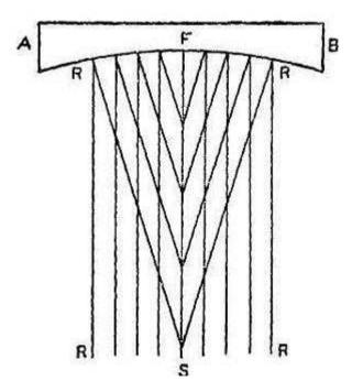
In the foregoing illustration let A-B be the mirror with F for its focus. Let the subject be stationed at S. Then the rays directed towards the surface of the mirror will be represented by RR-RR. These rays impinge upon a
